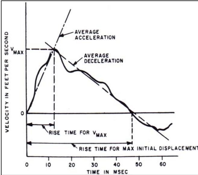
Figure 3: Example of shock-motion terminology [5].
