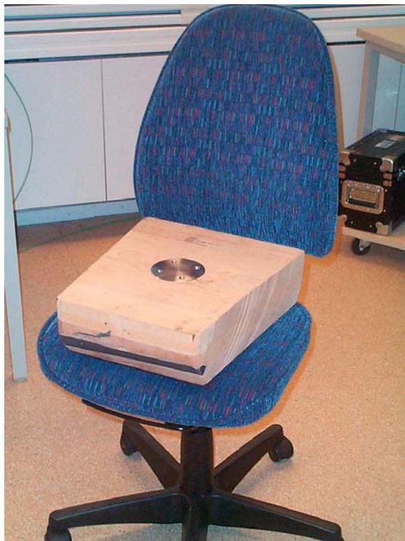
Figure 8: 10 kg wooden block with accelerometer mount.
